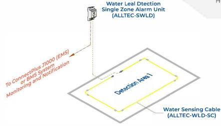
Water Leak Detection Single Zone Alarm Unit ALLTEC-SWLD
