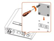
Plug the RJ45 connector into the "Meter" terminal and screw the shroud to the inverter.
