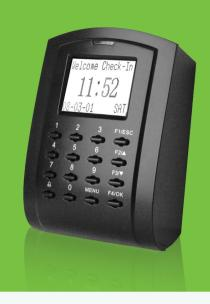
SC103 is an access control device produced by ZKTeco, which is made with elegant design and professional surface treatment. The device has lock control, alarm, exit, button and door sensor. The wiegand-in interface is used to connect external reader to construct master and slave system. Also, the device can be used to connect with a control panel as a
