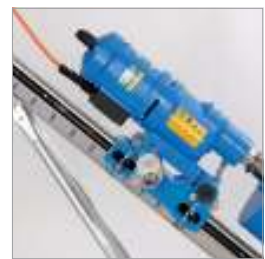
Simple drilling of diagonal holes using angle indicator
