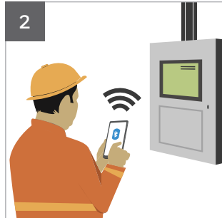
2 Establish a Bluetooth connectivity between mobile application and Fire Alarm Control panel.
